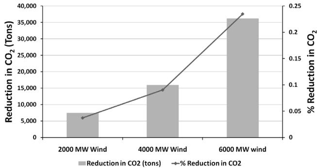
Fig. 1. Reduction in CO<sub>2</sub> emissions resulting from facilitation of multi-mode CCGT operation, shown for various generation portfolios
