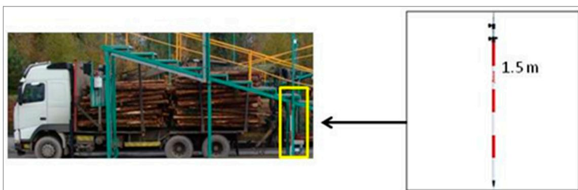
Figure 2. Location of the measuring staff for scaling.
