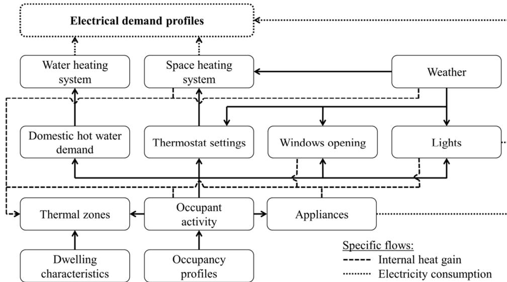
Figure 1: Bottom-up structure of building model
