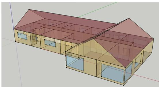
Figure 2: Single-storey detached house and thermal zones
