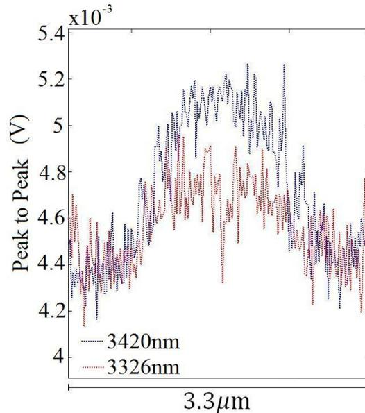
Fig. 5. Cantilever oscillation peak to peak voltages at IR absorption wavelengths tuned to resonance 3420nm (blue) and off of resonance 3326nm (red). A 56% reduction in signal is observed for the off resonance AFMIR.
