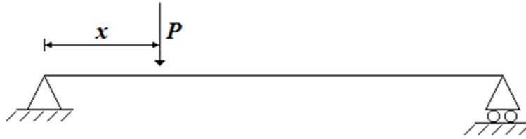
(a) Force at a fixed point,  $x$ , on the beam with  $P=100kN$ .
