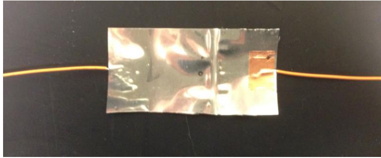
Figure 1. Image of PVDF Energy Harvester
