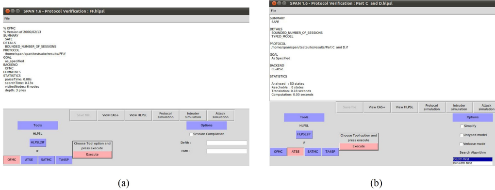
Figure 5.13: AVISPA outcome for Part C using (a) OFMC backend server (b) CL-Atse backend server
