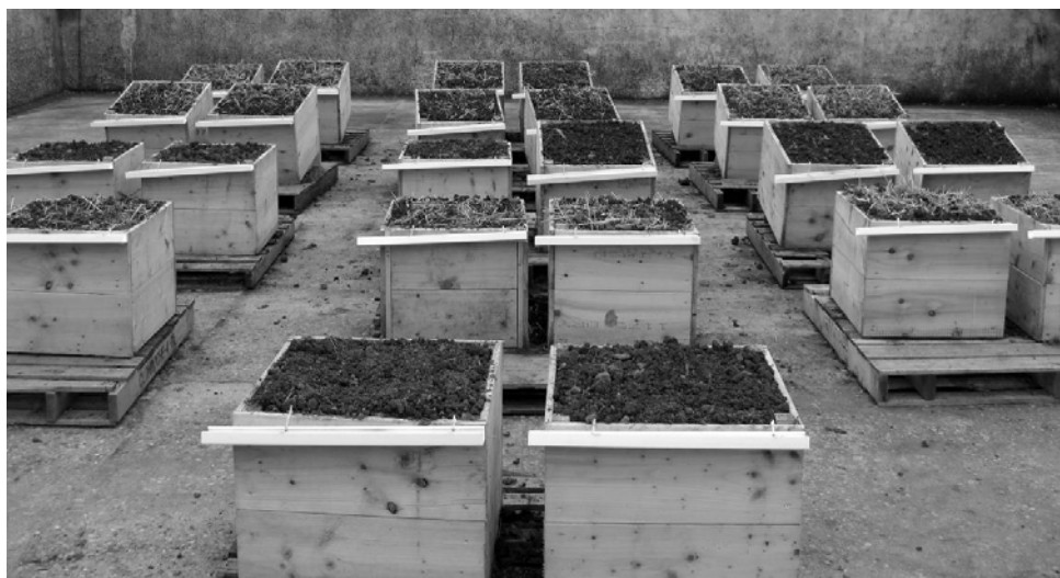
Figure 1: Soil boxes used to determine impact of fungal application to various soil/straw combinations at different slopes.
