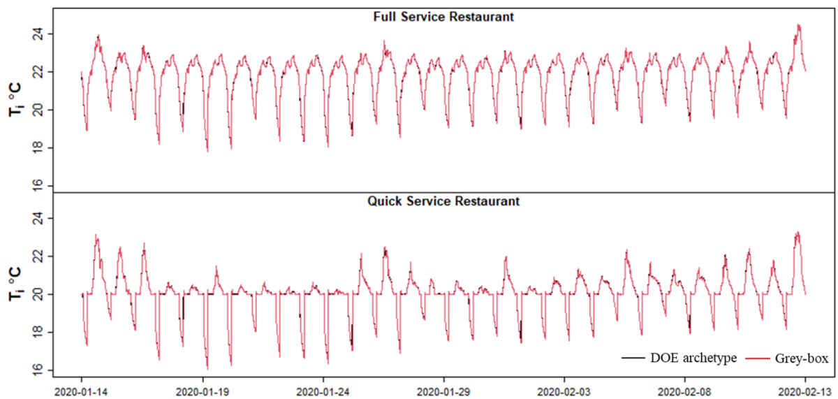
Figure Appendix B.3: Higher order model DOE archetype and grey-box internal temperature profiles for the full service and quick service restaurant DOE archetypes at the whole building level over a four week period.
