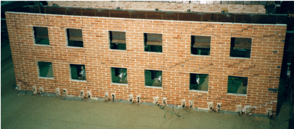
b) Test 5 at end of study (excavation from right side)
