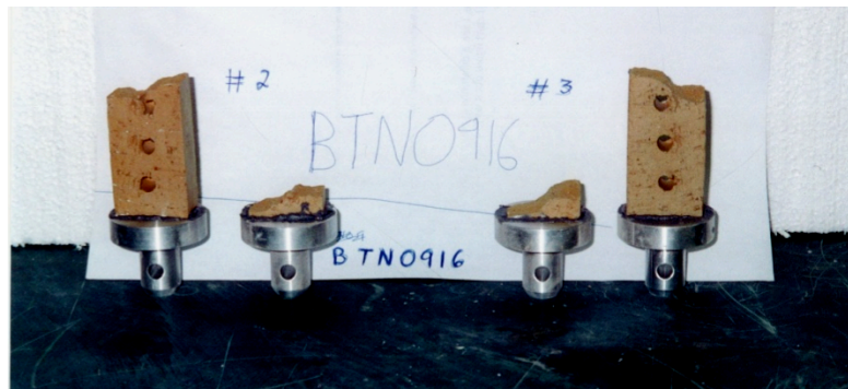
Fig. 12. Photograph of tensile brick testing.
