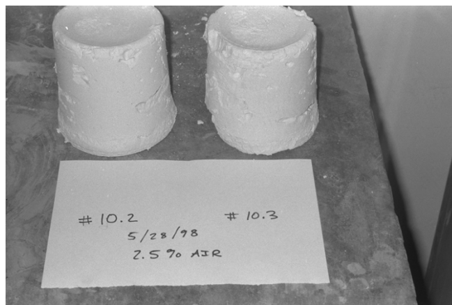
Fig. 7. Oversized cast mortar samples from which 5.1 cm x 5.1 cm samples were cut.
