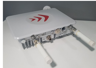
Fig. 2: 4G Base Station
