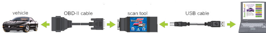
Figure 1: The engine control unit is connected through a serial cable to the scantool and a USB cable takes data to the laptop.
