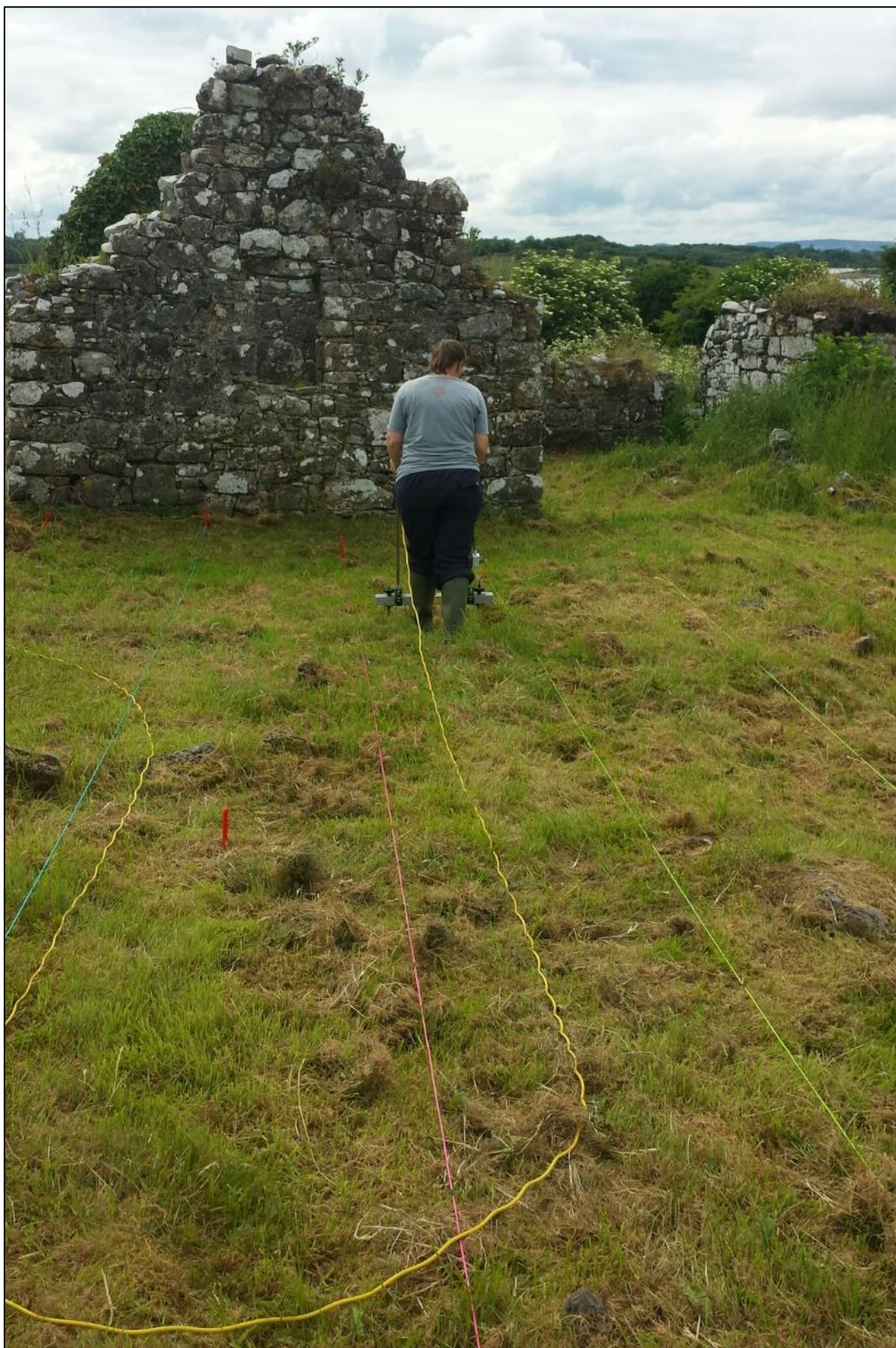
Figure 3.27 Undertaking the earth resistance survey at Tumna, Co. Roscommon (Photo: O. O'Rourke)
