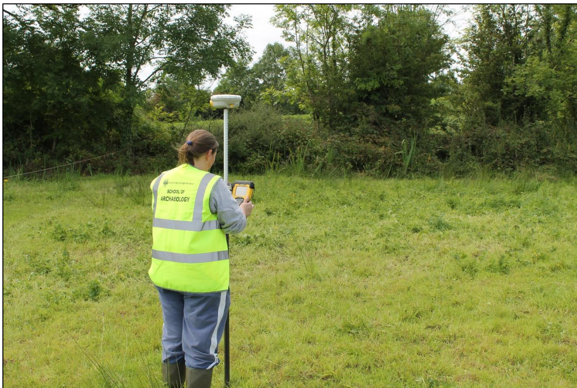
Figure 3.25 Setting out the geophysical survey grid points in the field with Trimble VRS Now GPS (Photo: O. O'Rourke)
