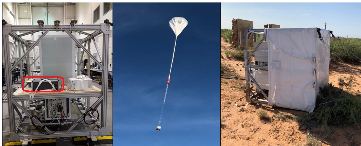
Figure 4.6: The balloon flight payload and gondola, from launch, ascent to landing. Left ) GMoDem secured to the gondola structure and highlighted for clarity. Center ) The balloon flight launch showing the zero pressure balloon, flight train and the payload. Right ) The gondola after landing.
