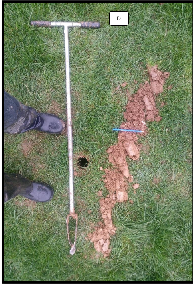
Figure 9-2. D) Stainless steel soil auger used for soil texture/drainage class assessment.
