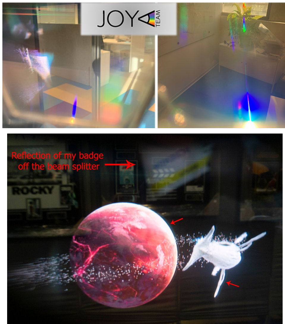
Figure 1. 6 Ghost images of augmented reality device [60]
