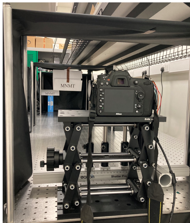
Figure 4. 46 Targets are set in the system for varifocal model. Two same letters are set at 100 cm and 200 cm away from the camera.
