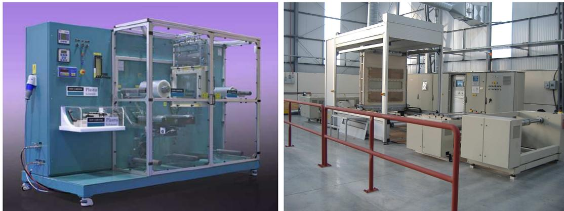
**Figure 2: LabLine & AP4 reel-to-reel atmospheric pressure plasma systems for the treatment of webs up to 0.3 and 1.2 Meters wide respectively**
