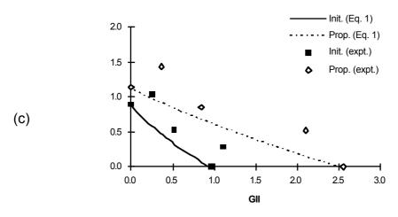
**Figure 24.** Initiation and propagation fracture toughness data as measured experimentally and predicted analytically using Eq. (1) [8] for the annealed woven material (a), the woven material (b) and the warp knitted material (c).
