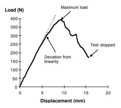
Figure 11. A typical load/displacement curve for a woven laminate tested in Mode II.
