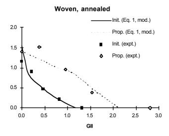
**Figure 25.** Experimental fracture toughness data and the predicted failure loci for the woven annealed material using a modified form of Charalambides' [8] criterion based on the experimentally assumed cusp angles [7] (compared against Fig. 24a).
