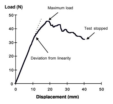
Figure 6. A typical load/displacement curve from a Mode I test of a warp knitted laminate.
