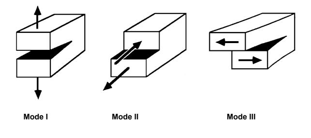
Figure 1. The three different crack propagation modes [1].
