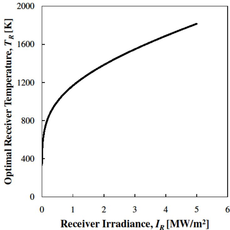
*Fig. 3. Optimal receiver temperature versus receiver irradiance*
