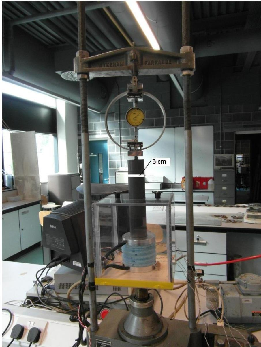
**Figure 2 UCD divided bar apparatus**
