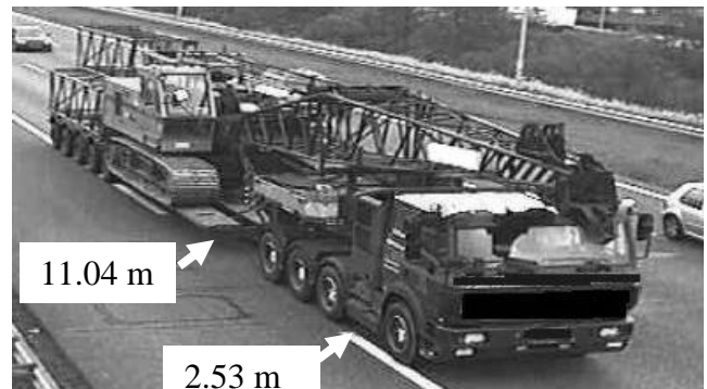
(b) GVW=100.8 t, wheelbase=22.3 m
