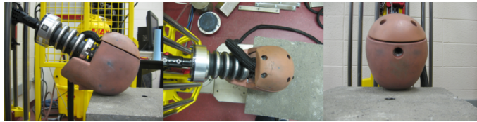
Figure 1. Hybrid III reconstruction of a fall.
