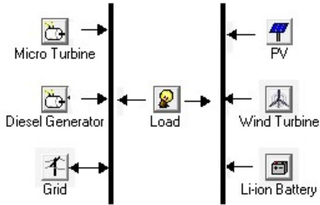
Figure 1: A typical schematic of the VPP.
