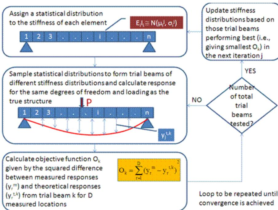
Fig. 1 – Cross-Entropy algorithm for estimation of stiffness distribution
