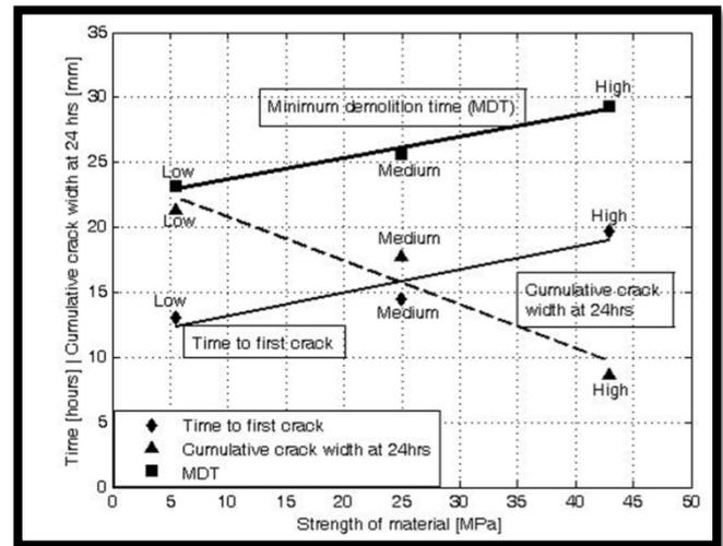
Figure 2: Crack patterns plotted against strength of material [16].
