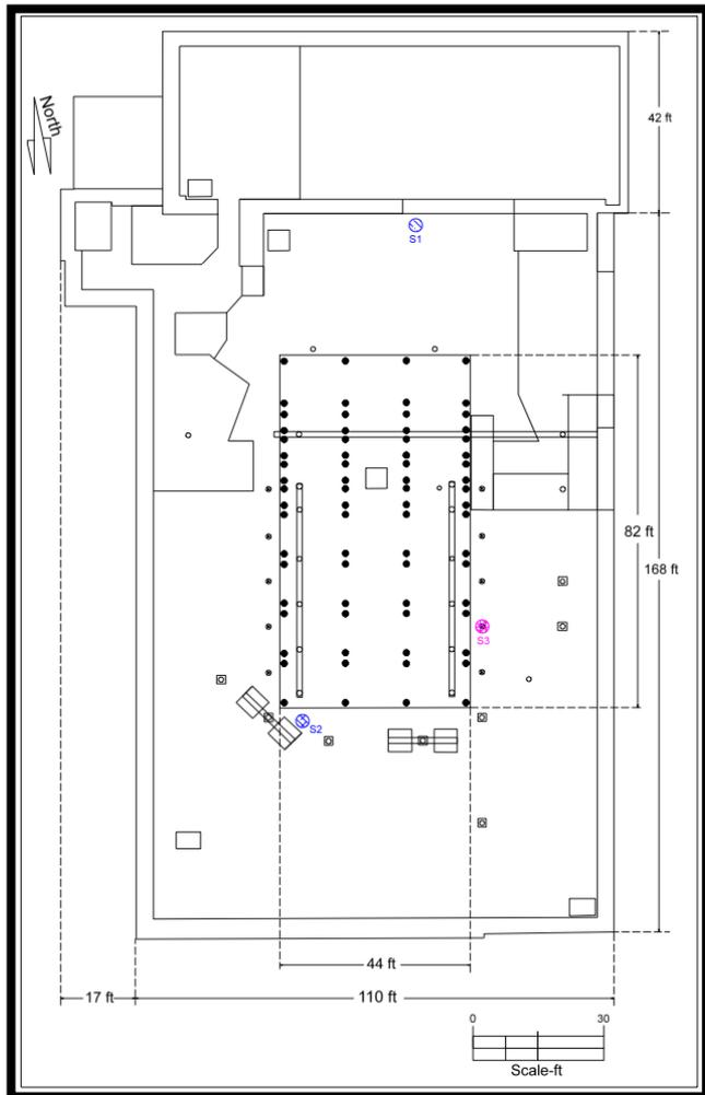
Figure 5: Plan of hall: S1, S2 and S3 are Seismographs. Bolded dots are temporary support steel columns.
