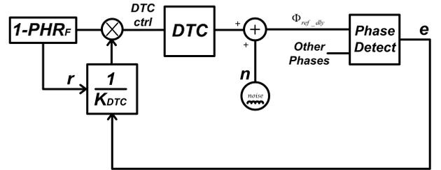
Fig. 4: Block diagram of DTC gain calibration.
