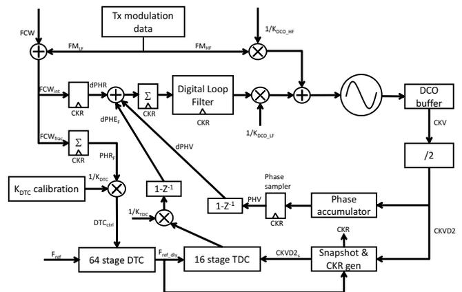
Fig. 1: DTC-based ADPLL architecture.
