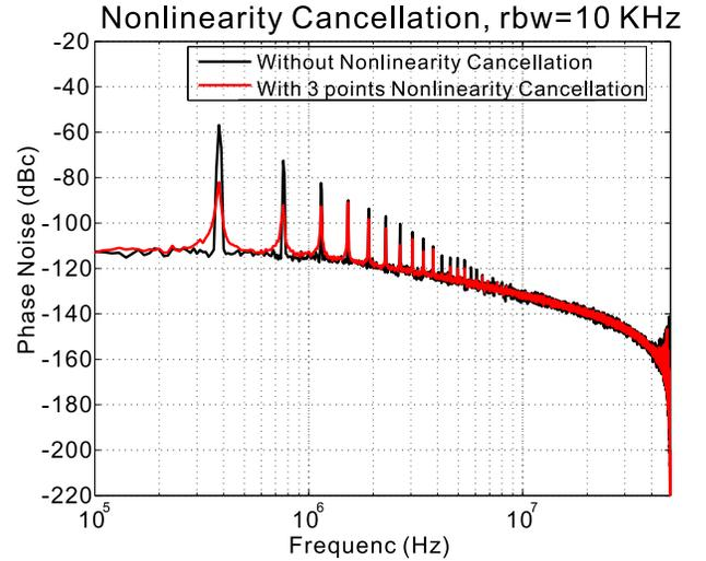
Fig. 7: Phase noise comparison with the 3-point nonlinearity cancellation.
