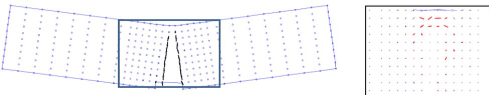
395 c- Crack pattern, exaggerated deflected shape, and principal stresses near mid-span at cycle
