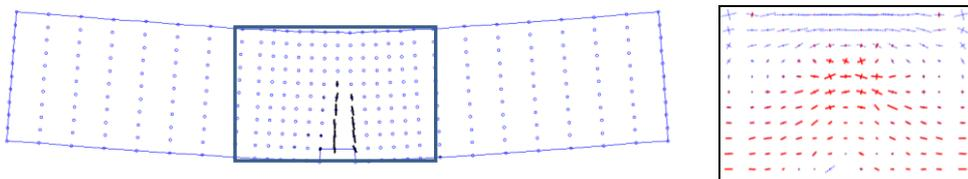
392 b- Crack pattern, exaggerated deflected shape, and principal stresses near mid-span at cycle
