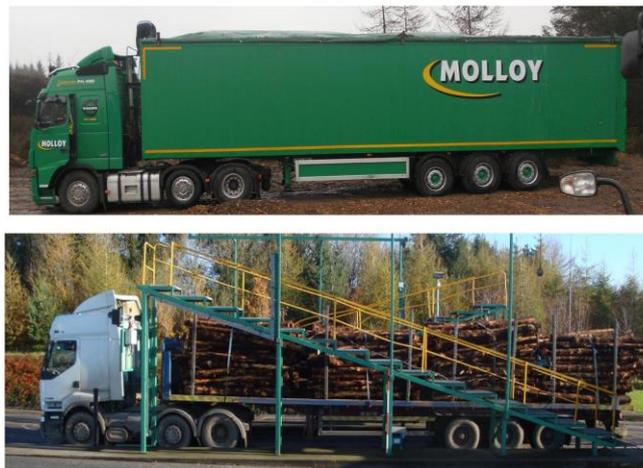
Figure 11 Truck types used to haulage wood chips and logs.
