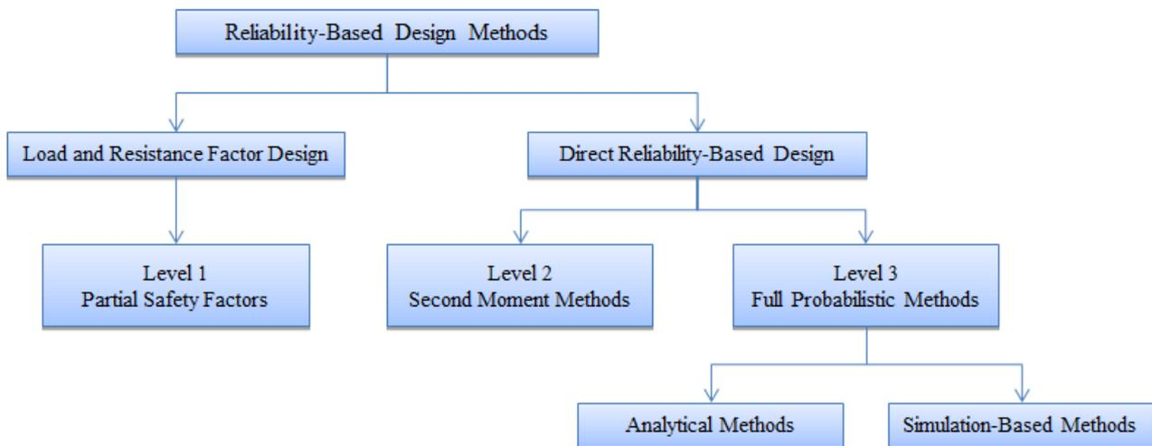
**Figure 3.** Levels of probability procedures for reliability-based design
