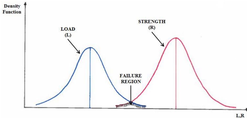
**Figure 4.** Frequency distribution of strength R and Loads L (Adapted from Ayyub and Assakkaf 2000)
