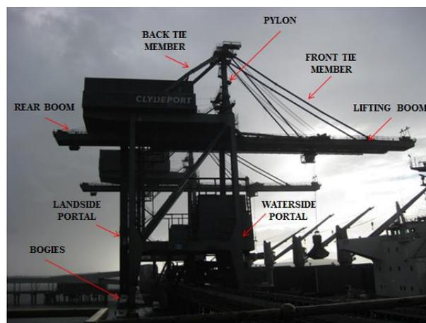
**Figure 1.** Ship unloader elements: Lower (Bogies, waterside portal, landside portal, hopper and diagonal brace) and Upper Substructures (Lifting boom, rear boom, front tie member, back tie member and pylon)
