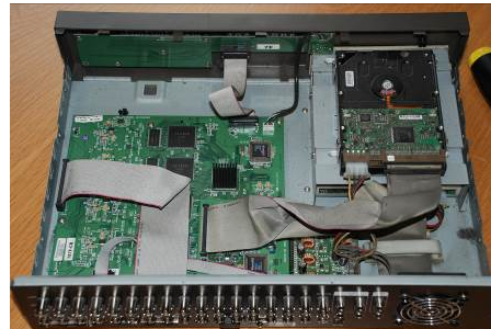
Figure 2: Internal view of the Ganz C-MPDVR-16 DVR unit.
