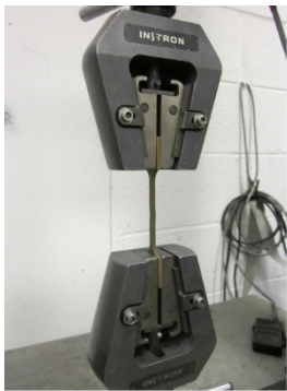
Figure 1: (a) - The tensile test procedure, (b) - True stress–strain curves obtained from tensile tests.
