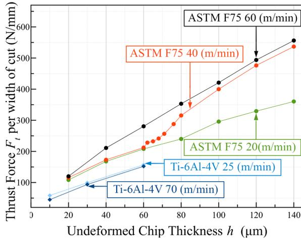
Figure 6: Thrust Force  $F_t$  per Width of Cut vs. Undeformed Chip Thickness.
