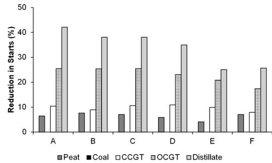
Fig. 6. Reduction in conventional plant starts (%) 15 minute resolution
