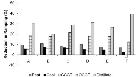
Fig. 7. Reduction in conventional plant ramping (%) 15 minute resolution
