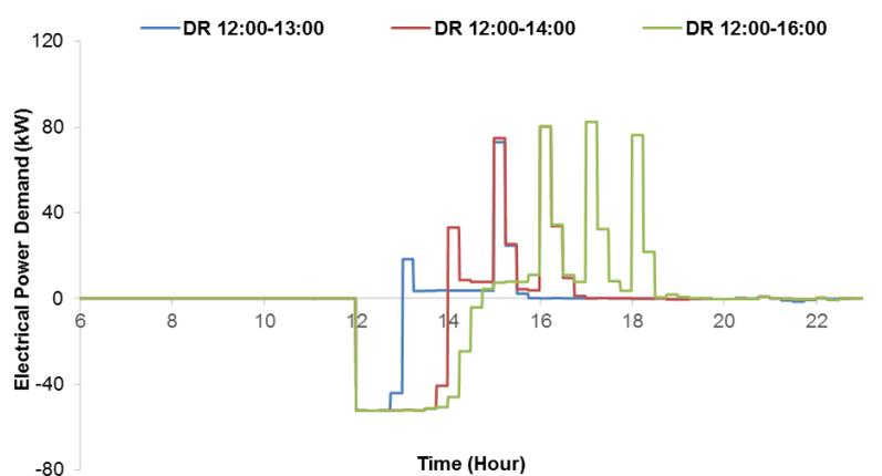
Figure 5: Difference in building electric load demand for the CWT strategy
