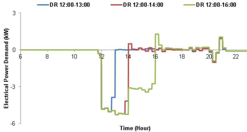
Figure 8: Difference in building electric load demand for the supply air flow rate decrease strategy
