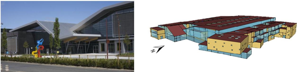
Figure 2: EnergyPlus building model of the Student Learning Leisure and Sports Facility (SLLS)
