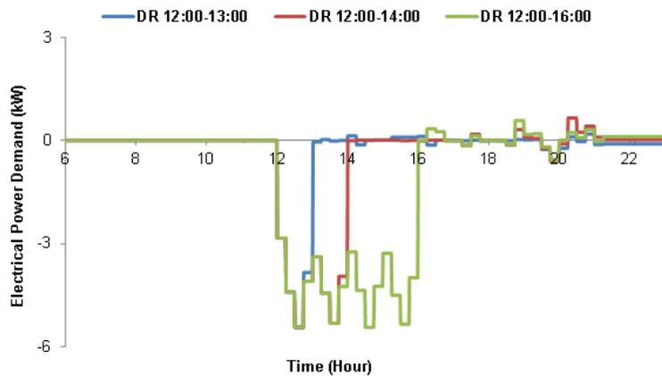
Figure 7: Difference in building electric load demand for the offices FCUs on / off control strategy
