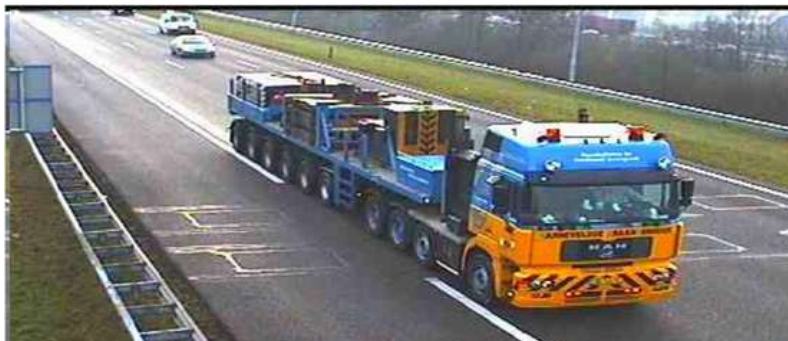
(c) Crane ballast truck (109 tonnes, 10 axles).
