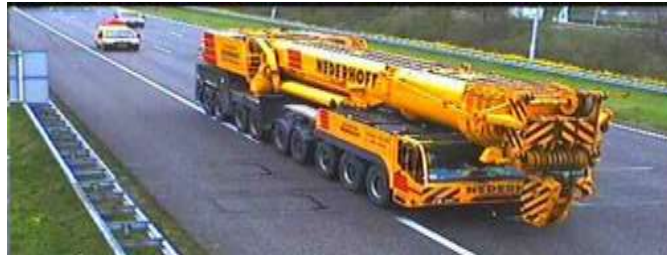
(a) Mobile crane (109 tonnes, 9 axles).
