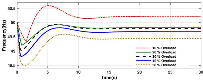
Figure 12. System frequency response using Decreasing UFLS
