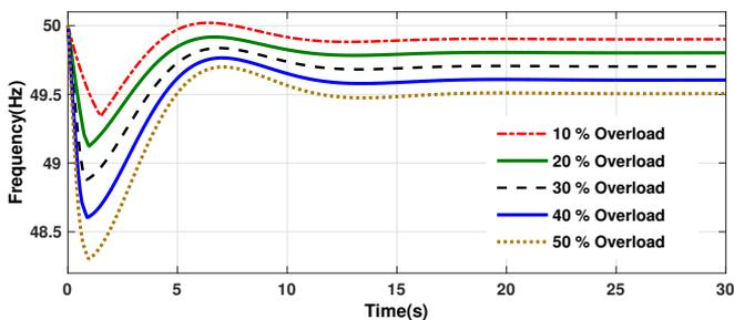
Figure 10. System frequency response using Equal Block UFLS plan
