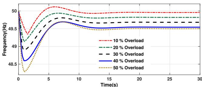
Figure 9. System frequency response using Sandwich UFLS plan
