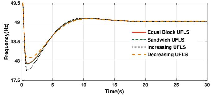
Figure 6. System frequency response using four UFLS strategies
