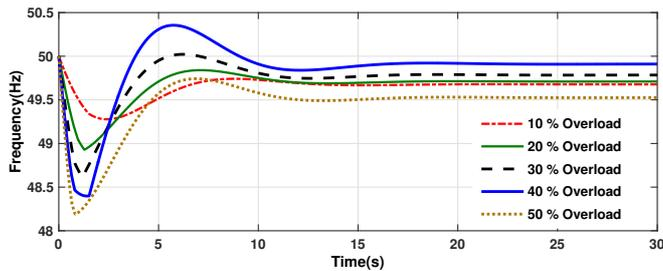
Figure 11. System frequency response using Increasing UFLS plan
