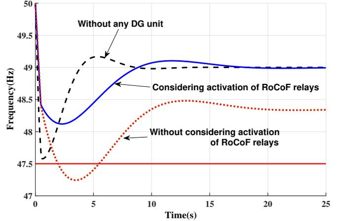
Figure 3. System frequency response using deterministic UFLS
