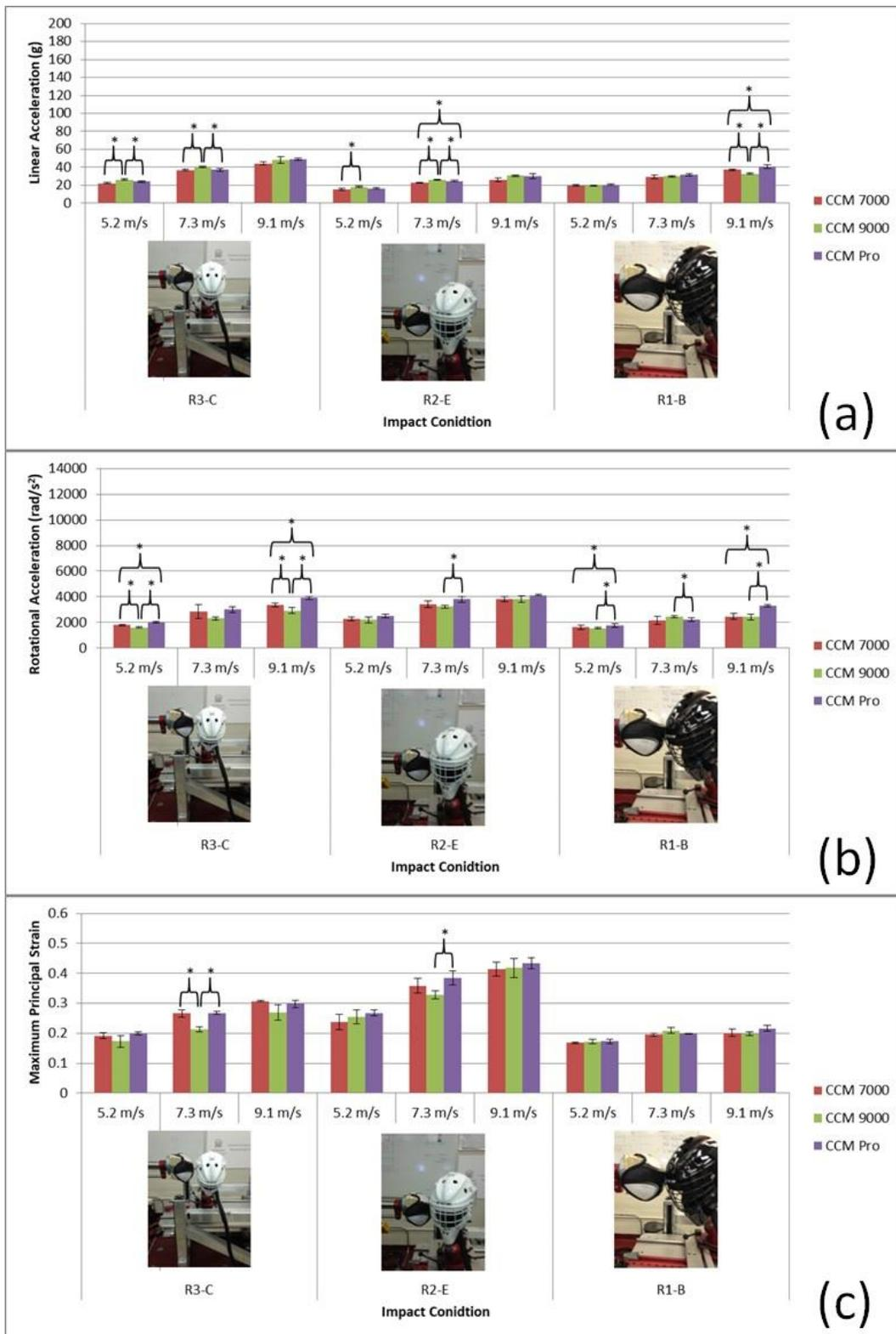
**Figure 8.** Mean peak kinematic response and maximum principal strain of collisions for three ice hockey goaltender helmets: (a) linear acceleration; (b) rotational acceleration; (c) maximum principal strain.
