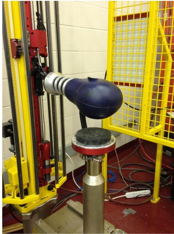
**Figure 4.** Monorail drop rig with NOCSAE headform attached.
