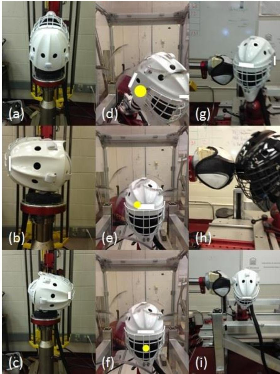
**Figure 3.** Impact location of an event specific impact test protocol for ice hockey goaltender helmets: (a) fall Rear-D, (b) fall L4-D, (c) fall R3-D, (d) puck impact Front-D, (e) puck impact R1-B, (f) puck impact R3-D, (g) collision R2-E, (h) collision R1-B, (i) collision R3-C.<sup>4</sup>
