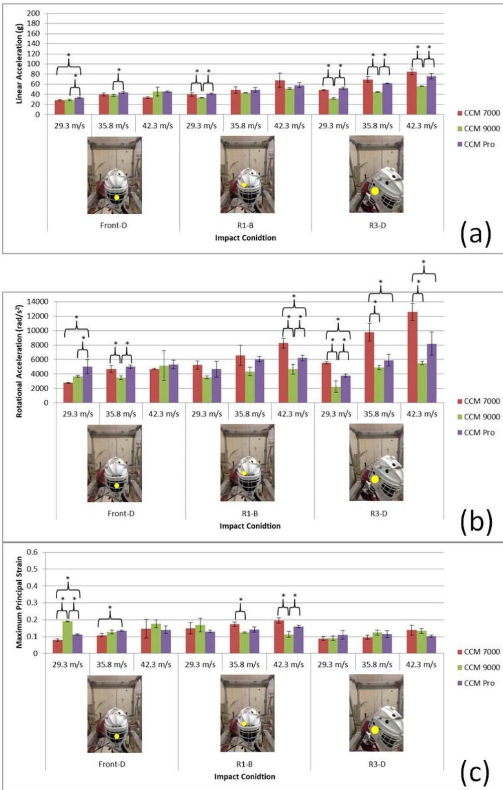
**Figure 7.** Mean peak kinematic response and maximum principal strain of puck impacts for three ice hockey goaltender helmets: (a) linear acceleration; (b) rotational acceleration; (c) maximum principal strain.
