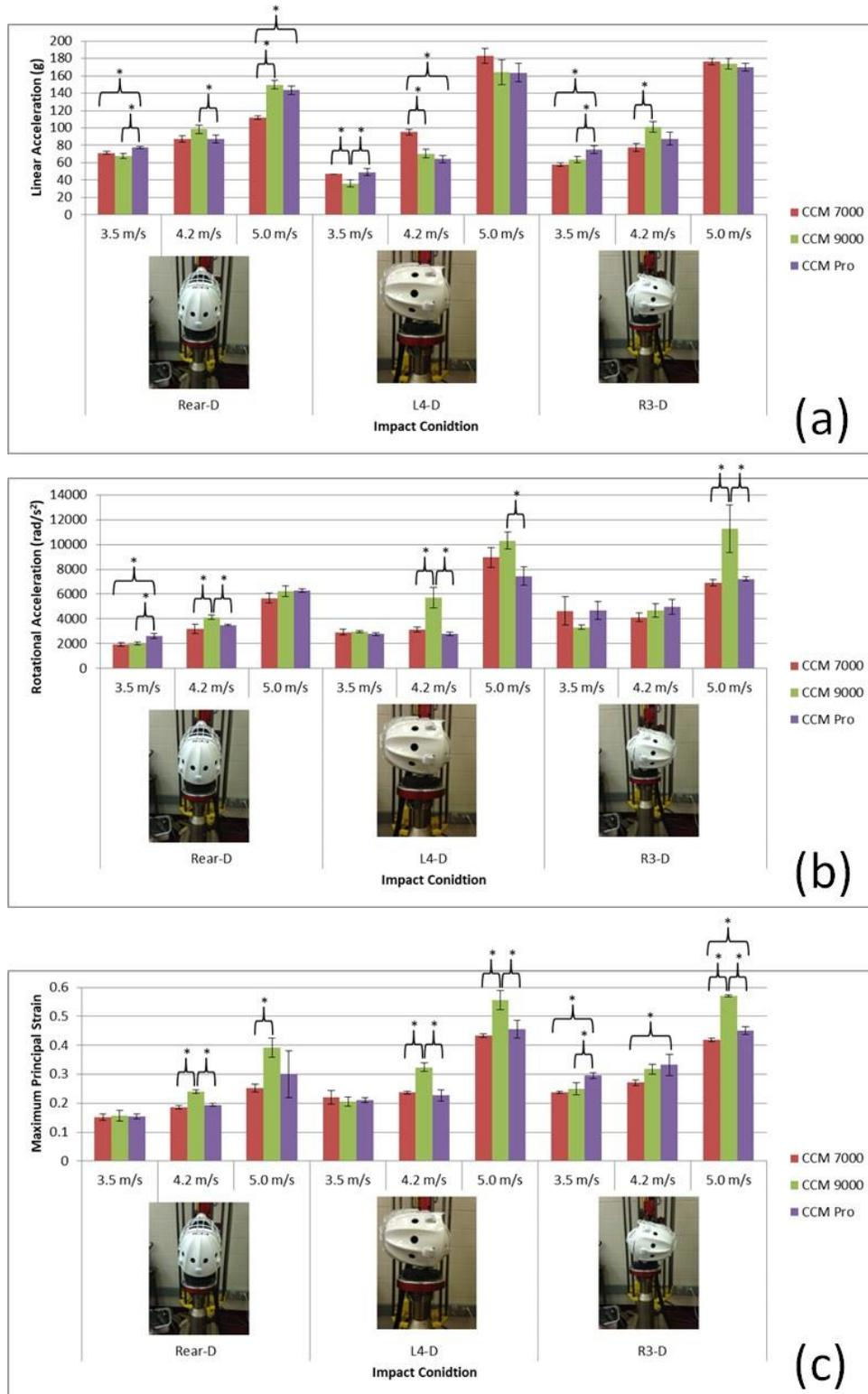
**Figure 6.** Mean peak kinematic response and maximum principal strain of falls for three ice hockey goaltender helmets: (a) linear acceleration; (b) rotational acceleration; (c) maximum principal strain.
