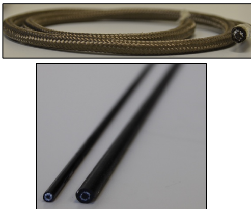
Figure 1. (a) BFRP rebar preform, (b) Resin impregnated composite rebars.
