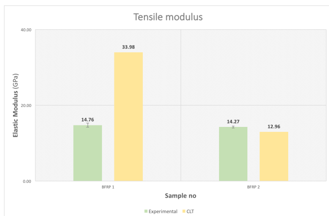
Figure 5. Tensile modulus of elasticity ( E_x^{FRP} ) for the two different rebar designs - Experimental vs CLT results.
