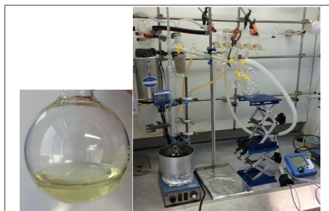
Figure 3 Distillate from 1 st distillation and set-up for second distillation of isothiocineole 1.
