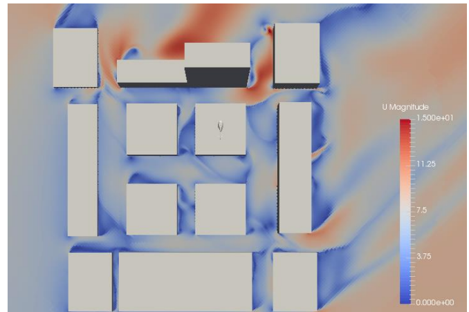
Fig 6 : Velocity Contour at 1.6 m AGL for a built environment with a non operating helicopter
