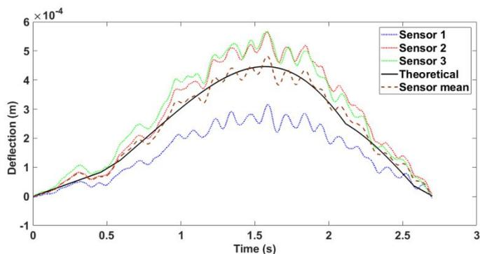
Figure 6. Comparison between theoretical deflection assuming a healthy bridge and the real measurements.
