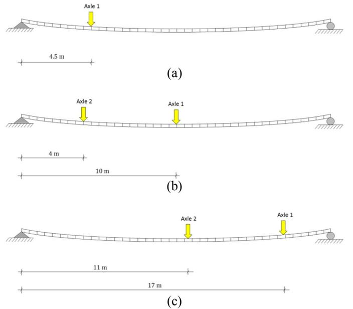
Figure 3. Load cases for sensitivity analysis when (a) 1<sup>st</sup> axle is at 4.5 m, (b) 1<sup>st</sup> axle is at mid-span and (c) 1<sup>st</sup> axle is at 17 m.
