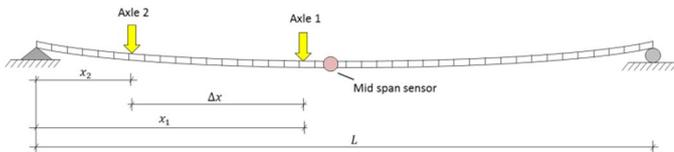
Figure 1. Beam model with two loads.
