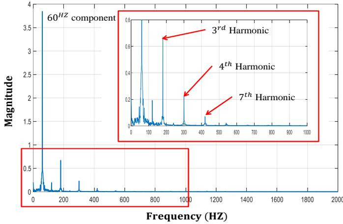
Fig. 7. Frequency components of simulated HIF current
