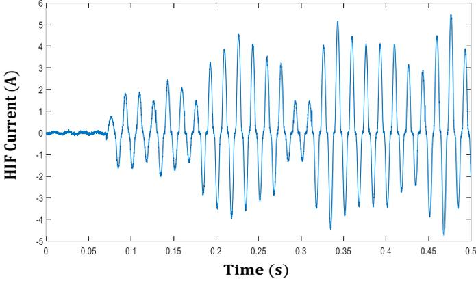
Fig. 6. Fault current using modified Emanuel HIF model
