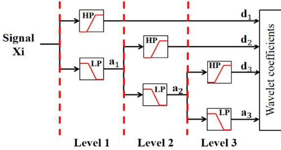
Fig. 2. Decomposing signal using DWT
