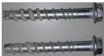
Figure 3. Crushed materials in between the threads after PSP test.
