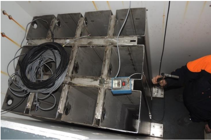
Figure 5. Hammer tests on the rack mock-up
