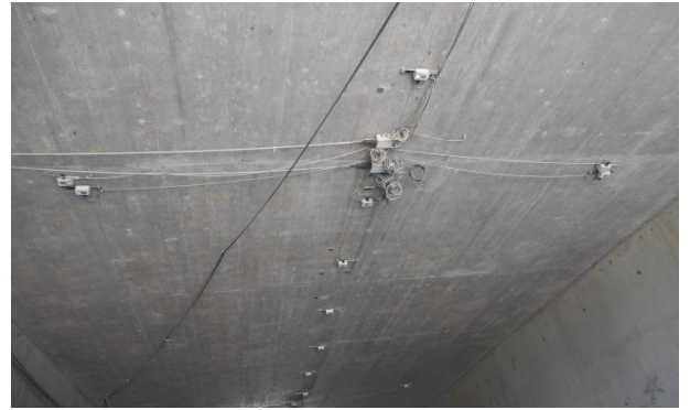
Figure 2. View of the strain sensors attached to the bottom of the slab of the case study bridge.
