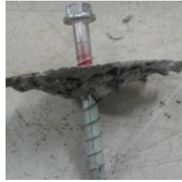
Figure 1b. Concrete cone failure.
