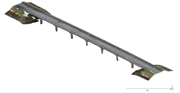
b. Point cloud after automatic noise removal
