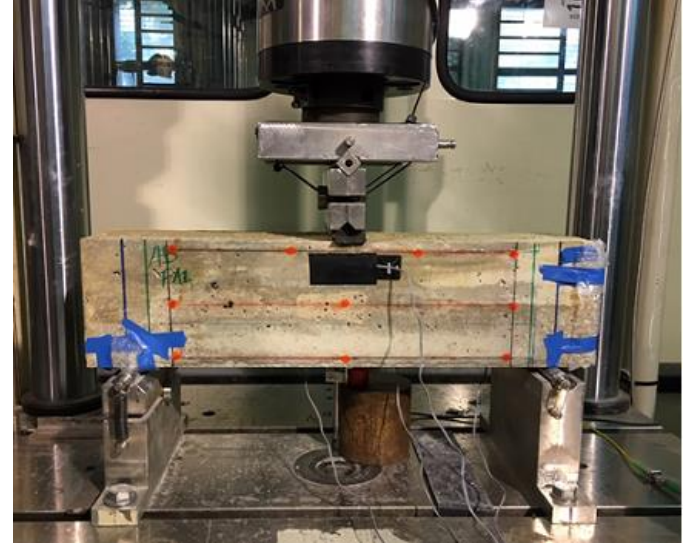
Figure 5. Load arrangement on tested reinforced concrete beam.
