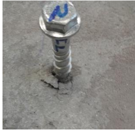
Figure 1a. Complete pullout failure.
