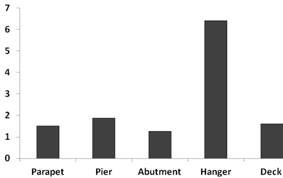
Figure 10. Empirical calibrations between HCP and resistivity of different component of bridges under consideration obtained in percentile mV/ percentile kΩ.cm.
