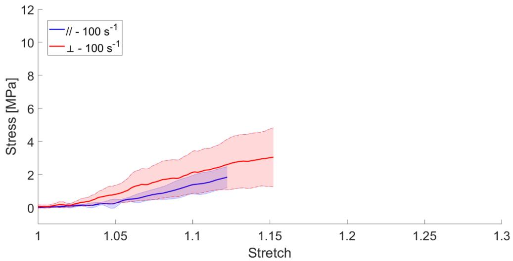
Figure. A. 6: Tensile tests performed on human scalp at a strain rate of  $100 \text{ s}^{-1}$ . The graph shows the average (continuous line) and the standard deviation (shaded area) for specimens parallel (in blue) and perpendicular (in red) with respect to the STLs.
