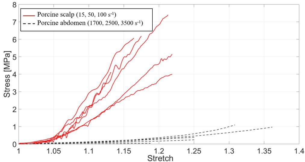
Figure 13: Comparison between tensile tests performed at high speed on porcine scalp (in red) and porcine skin from the abdominal area (dashed black line). Data for porcine skin from the abdominal area was reproduced from Lim et al. [62]. Results are shown in terms of Cauchy stress and stretch.
