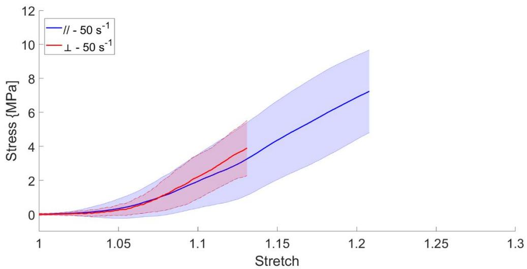
Figure. A. 2: Tensile tests performed on porcine scalp at a strain rate of  $50 \text{ s}^{-1}$ . The graph shows the average (continuous line) and the standard deviation (shaded area) for specimens parallel (in blue) and perpendicular (in red) with respect to the STLs.
