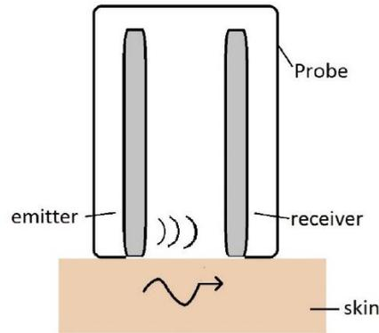
Figure 2: Basic schematic representing how the Reviscometer RVM 600 works. The emitter releases an acoustic wave and the receiver measures the RRT (Resonance Running Time). The direction of lowest RRT indicates the orientation of skin tension lines. Reproduced from Deroy et al. [43].
