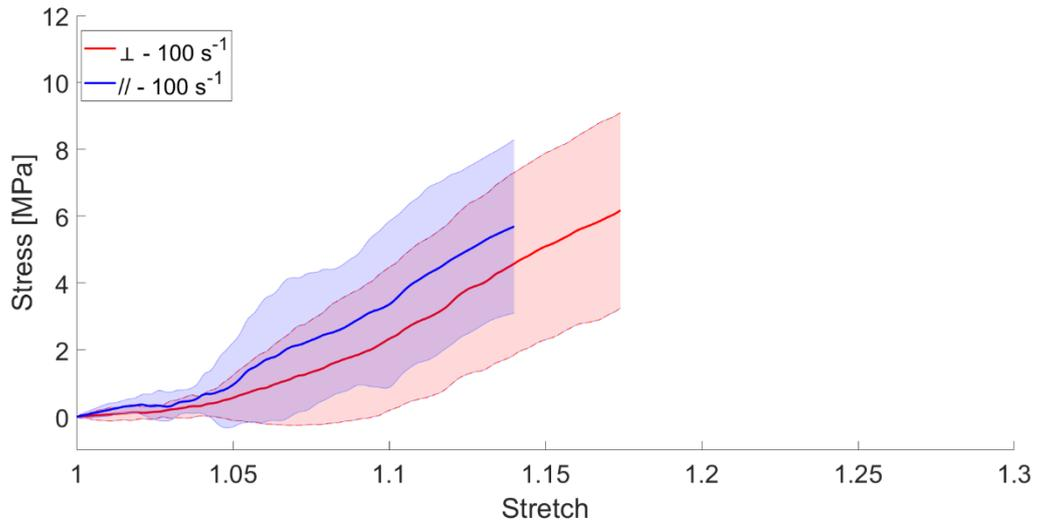
Figure. A. 3: Tensile tests performed on porcine scalp at a strain rate of  $100 \text{ s}^{-1}$ . The graph shows the average (continuous line) and the standard deviation (shaded area) for specimens parallel (in blue) and perpendicular (in red) with respect to the STLs.
