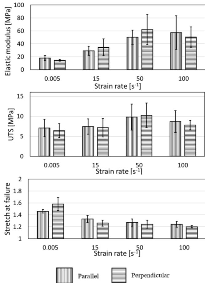
Figure 8: Bar chart of the average elastic modulus, UTS and the stretch at failure of porcine scalp at different strain rates. The error bar represents the standard deviation.
