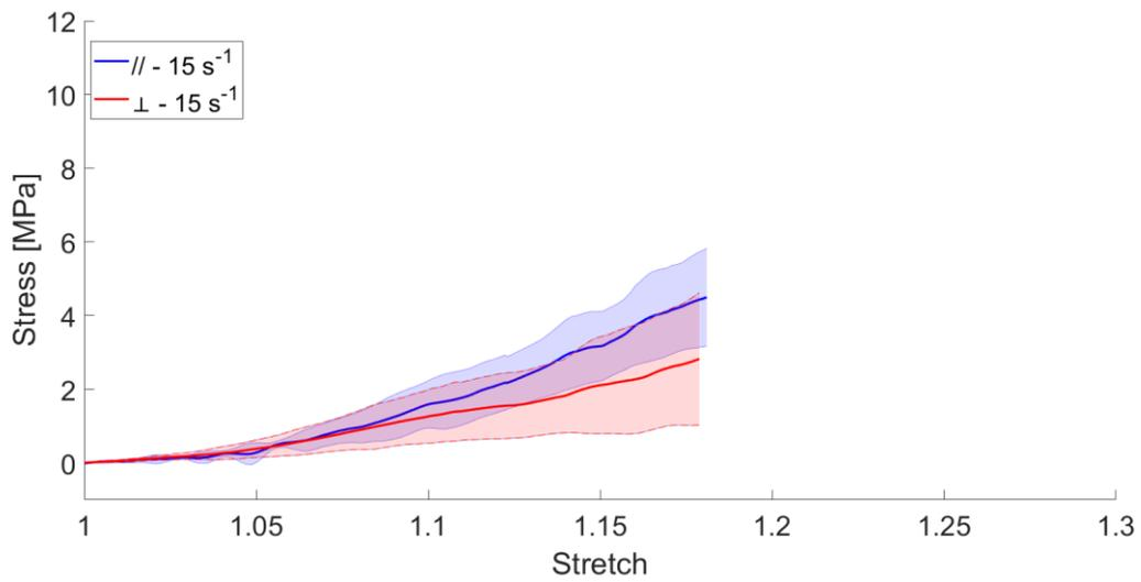
Figure. A. 4: Tensile tests performed on human scalp at a strain rate of  $15 \text{ s}^{-1}$ . The graph shows the average (continuous line) and the standard deviation (shaded area) for specimens parallel (in blue) and perpendicular (in red) with respect to the STLs.
