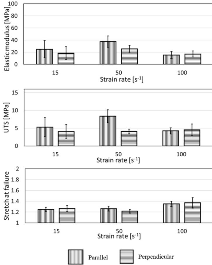
Figure 10: Bar chart of the average elastic modulus, UTS and the stretch at failure of human scalp at different strain rates. The error bar represents the standard deviation.
