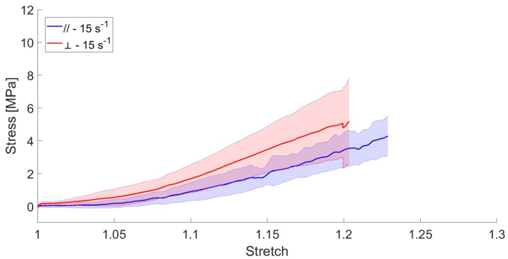
Figure. A. 1: Tensile tests performed on porcine scalp at a strain rate of  $15 \text{ s}^{-1}$ . The graph shows the average (continuous line) and the standard deviation (shaded area) for specimens parallel (in blue) and perpendicular (in red) with respect to the STLs.
