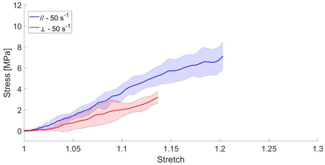
Figure. A. 5: Tensile tests performed on human scalp at a strain rate of  $50 \text{ s}^{-1}$ . The graph shows the average (continuous line) and the standard deviation (shaded area) for specimens parallel (in blue) and perpendicular (in red) with respect to the STLs.
