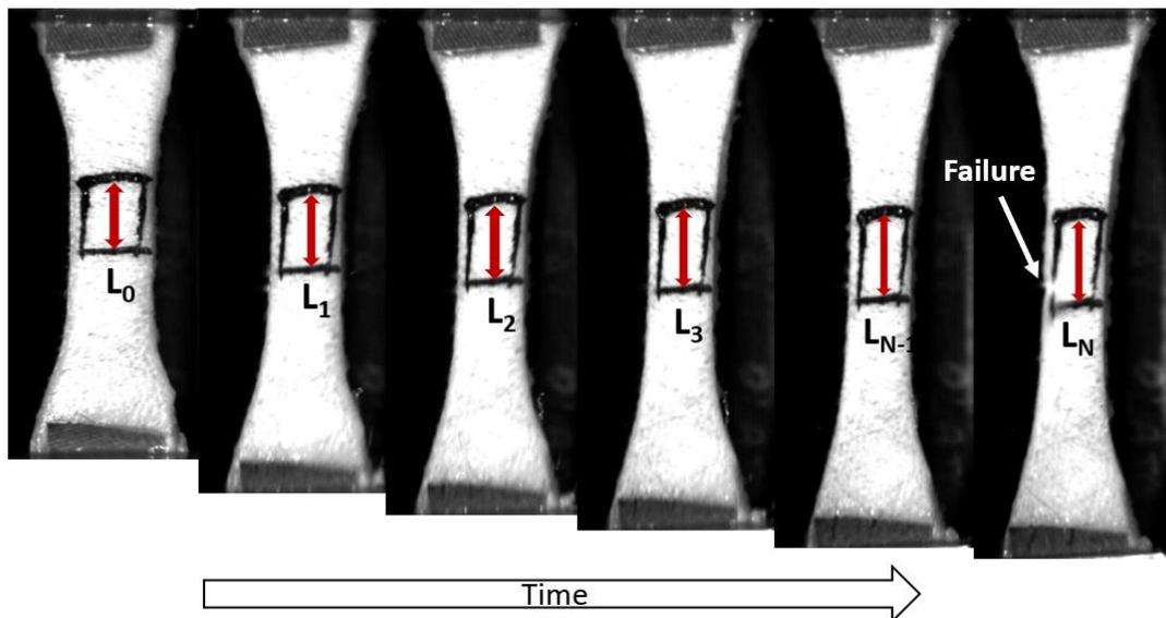
Figure 5: Stretch of the specimen determined as the ratio between the distance of two horizontal lines drawn on the sample at each time step and the initial distance,  $L_0$ .
