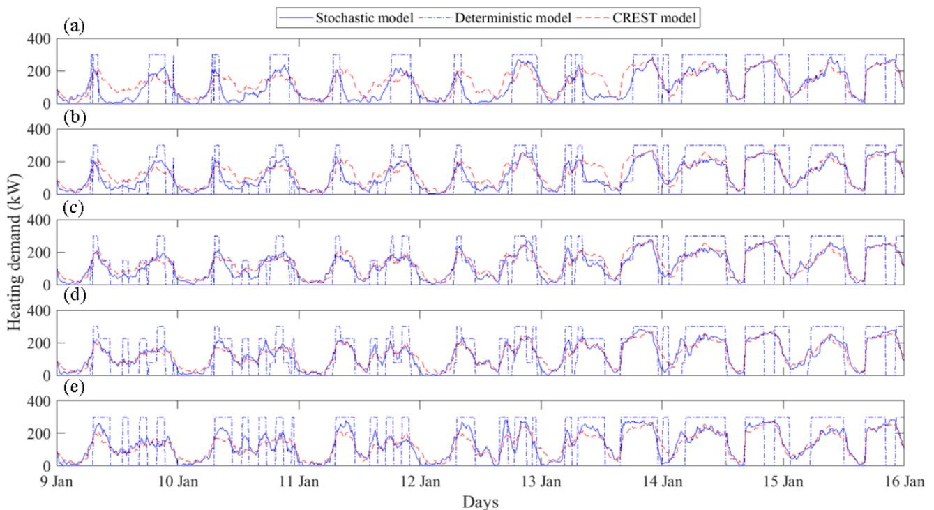
**Figure 21** Multi-day heating power load of the building stock (100 archetypes) from Jan 9<sup>th</sup> to Jan 15<sup>th</sup> 2012 for the following cases: (a) 100% OP2; (b) 75% OP2 – 25% OP5; (c) 50% OP2 – 50% OP5; (d) 25% OP2 – 75% OP5; (e) 100% OP5.
