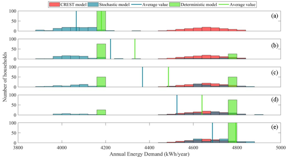
**Figure 16** Distribution of annual heating energy consumption of the modelled building stock for the following cases: (a) 100% OP2; (b) 75% OP2 – 25% OP5; (c) 50% OP2 – 50% OP5; (d) 25% OP2 – 75% OP5; (e) 100% OP5.
