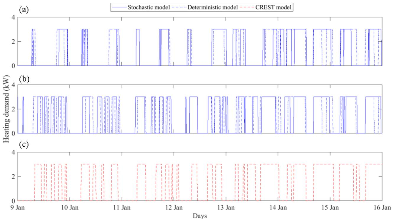
Figure 20 Multi-day heating power load of individual archetypes from Jan 9<sup>th</sup> to Jan 15<sup>th</sup> 2012 for the following cases: (a) archetype characterised by OP2; (b) archetype characterised by OP5; (c) no OP.
