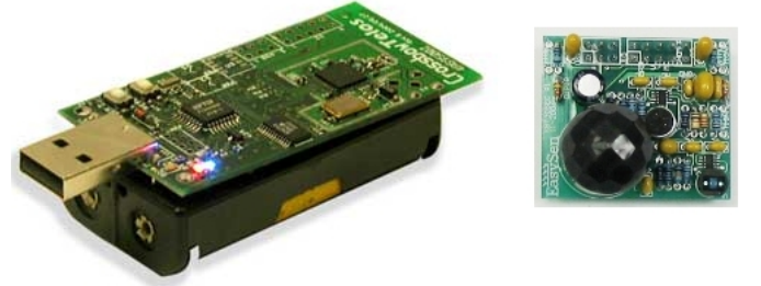
Figure 4. Crossbow telosb mote and EasySen sensor board
