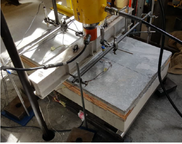
Figure 2. Precast concrete sandwich panel in a flexural test set-up
