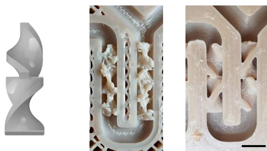
Figure 3. (Left) Intended internal mixer design (Centre) Printed mixer elements with 0.4 mm nozzle, 0.42 mm profile, 3 mm diameter (Right) Printed mixer elements with 0.4 mm nozzle, 1.2 mm profile, 4 mm diameter. Scale bar, for images in centre and right of figure only, is 5 mm.
