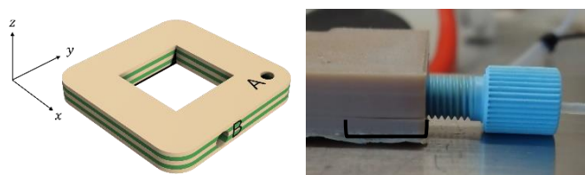
Figure 2. (Left) For the print orientation shown holes located at the position indicated by port B will result in layer separation on insertion of the threaded screw, this was not found when port A positioning with design shown in figure 1 was used. (Right) The effect of ports printed with a perpendicular profile to the build plane (extent of crack in reactor wall indicated).
