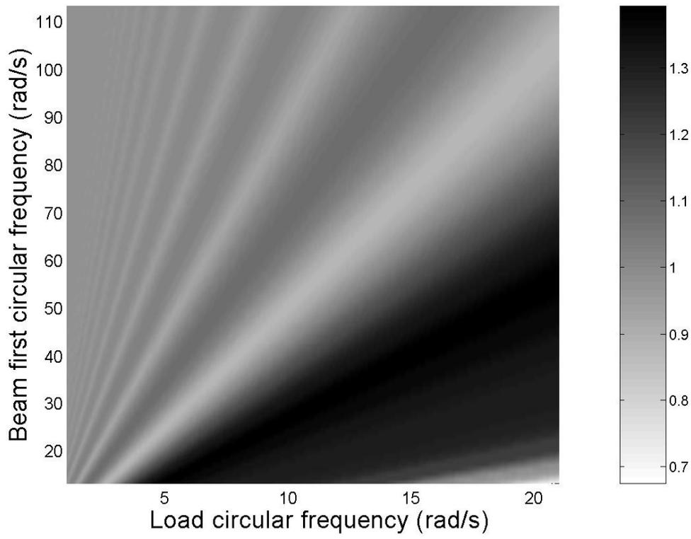
Figure 2 - Contour plot of amplification factor versus beam first circular frequency and load circular frequency (3 % damping)
