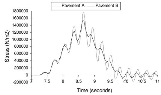
(b) - Effect of pavement profiles on dynamic response for two-axle vehicle in
