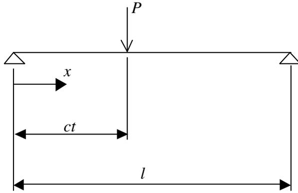
Figure 1 – Schematic of beam and load model
